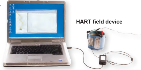
Windows®-based PC USB HART modem HART field device
